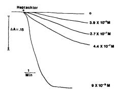
Figure 2. Effect of the concentration of heptachlor on light scattering.
